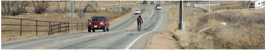
Insufficient shoulder width for multimodal use
